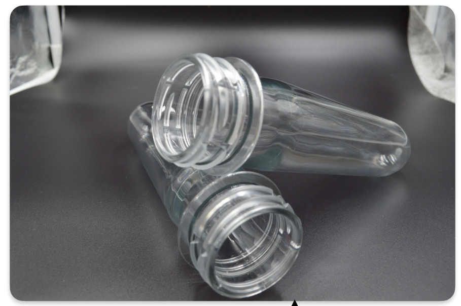
02 Injection machine will be fed the dried&crystallized rPET Pellets and make the Preform
